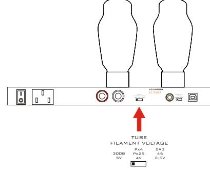
TUBE FILAMENT VOLTAGE
